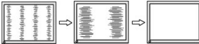
4. After adjusting the Clock, if blurring, flickering, or bars appear on the screen, proceed to adjust the Phase.
