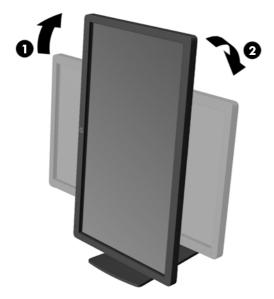
NOTE: To view information on the screen in portrait mode, you can install the HP Display Assistant software included on the software and documentation disc. The position of the OSD menu can also be rotated to portrait mode. To rotate the OSD menu, access the OSD menu by pressing the Menu button on the front panel, select **OSD Control** from the menu, then select **Rotate OSD**.
