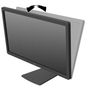
2. Swivel the monitor to the left or right for the best viewing angle.
