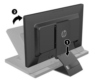
**NOTE:** When the monitor is unfolded for the first time, the display head is locked from adjusting to a full-height position. To adjust the display head to full height, press down on the display head to unlock it then pull up on the display head to raise it to the full-height position. Refer to step 3 in <u>Adjusting the Monitor on page 10</u>.
