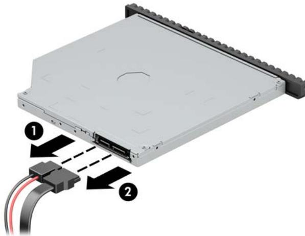
7. Press the release lever on the back of the drive (1), and then slide the drive through the front bezel (2).
