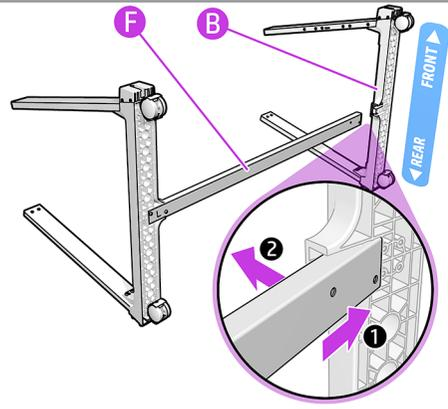
Insert the Bottom cross tube (F) diagonally into the right bottom connector (B).
