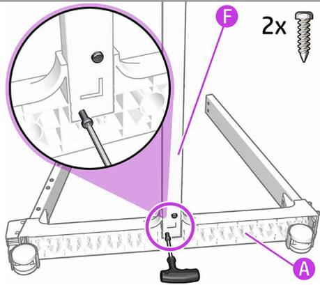
Fix the Bottom cross tube (F) to the Left Bottom Cross Connector (A) with two T25 screws.
