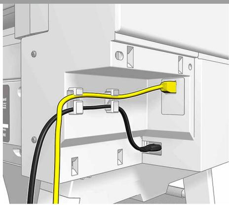
Route the ethernet cable and power cable through the cable clips.
