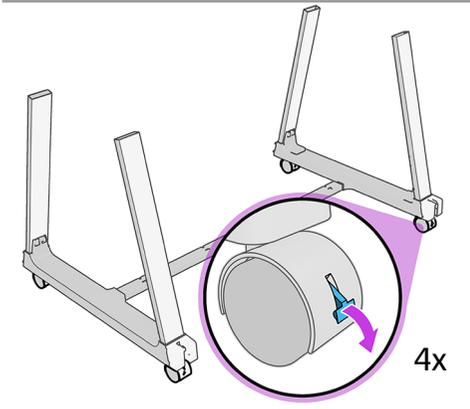
Place the stand upright and check the four wheels are locked.
