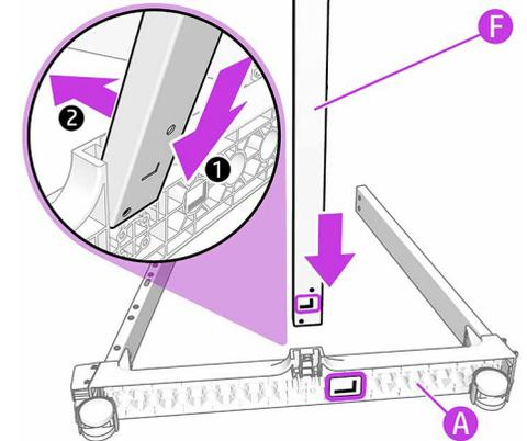
**Important:** Note the position of the holes on the left bottom cross-connector (A).
