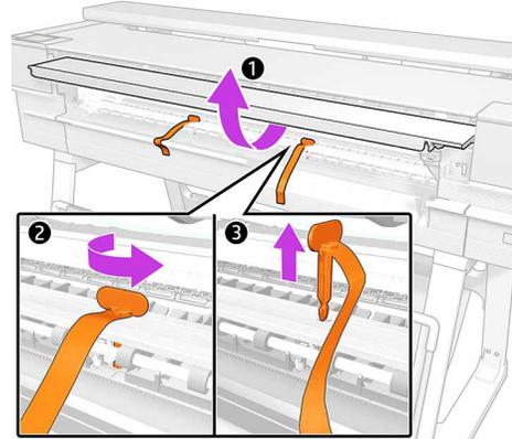
Open the main door. Carefully, rotate and remove the two pins from inside of the printer.
