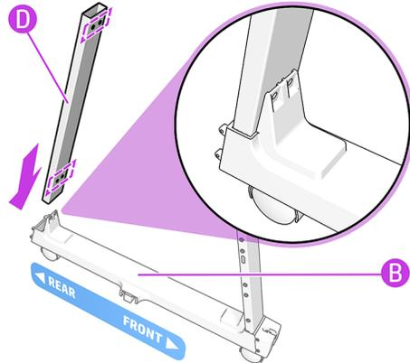
Insert the right rear-leg (D) onto the rear of the right-bottom cross-connector (B).
