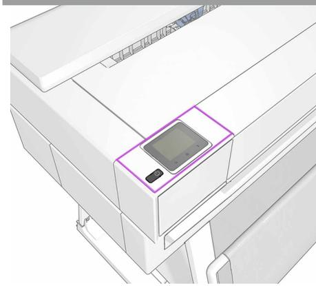
**Note:** Make sure all the covers are closed before power on the printer. Once all the cables are connected, check that the printer is on. The control panel will now guide you through setup.
