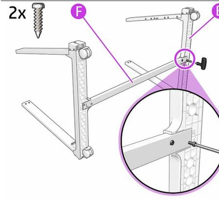
Fix the Bottom cross tube (F) to the right connector (B) with two T25 screws.
