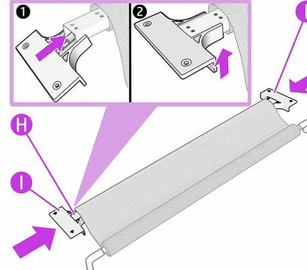
Diagonally insert the left and right brackets (I) to the rear cross-tube (H) by pushing them into place.
