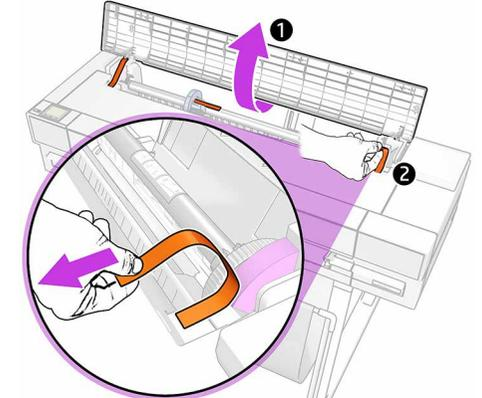
Open the roll cover and remove the two spindle tapes.
