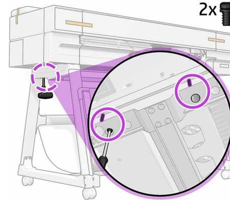
From underneath, fix the left side of the printer to the stand with two T25 screws. **Note:** There are marks on the printer that indicate the position of the screws.
