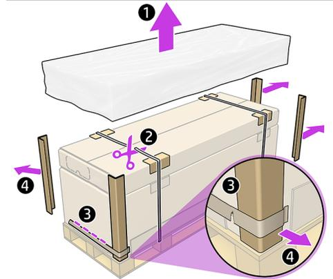
Remove the protective sheet (1), cut the straps (2), take off the corner protectors (3/4)
