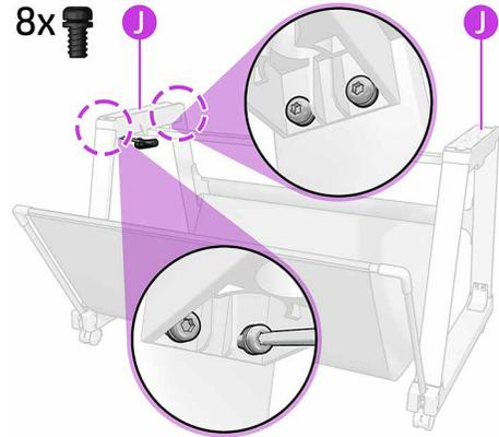
Fix the top cross-beam (J) to the stand with four T25 screws on the **left and right side**.
