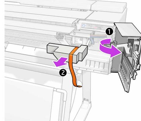
Open the printhead carriage door and remove the foam and close back.
