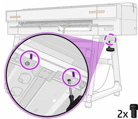
From underneath, fix the right side of the printer to the stand with two T25 screws. **Note:** There are marks on the printer that indicate the position of the screws.
