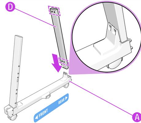
Insert the left rear-leg (D) onto the rear of the left bottom cross-connector (A).
