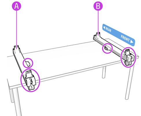
**HP recommends completing the assembly on a table.** Remove the 2x Bottom Cross Connectors (A and B) from the box.
