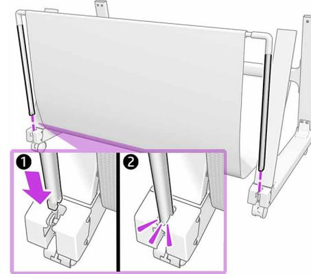
Insert the tubes into the slots at the front of both bottom cross-connectors. Push them firmly into place until you hear a click.
