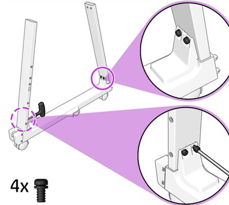
Fix the legs in place with two T25 screws each side.
