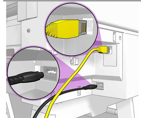
Connect a LAN cable (not included). Connect the power cable.
