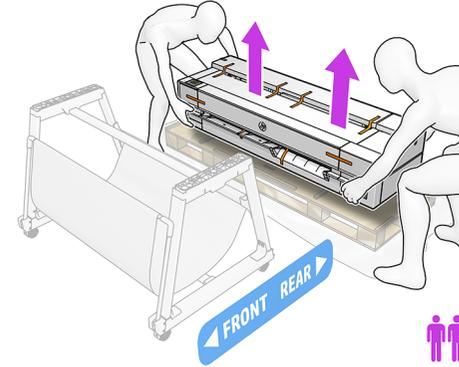
**Important:** Two people are required. Move the printer close to the stand, then with two people; lift the printer body by holding the base.
