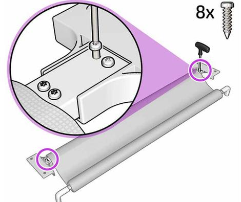
Fix the brackets in place with four T25 screws each side.
