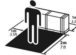
To ensure an accessible operating area for printer use, it is recommended to leave a minimum clear space of 760 mm (30 inches) by 1220 mm (48 inches) with an even level around the sides of the printer. Light reflection (glare) could affect the readability of the control panel, to improve the visibility, select the most suitable theme (dark-light) in the Control Panel.
