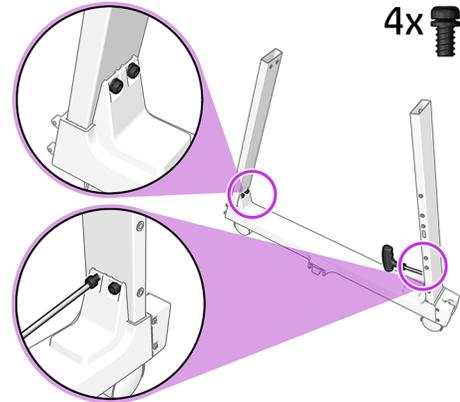
Fix the legs in place with two T25 screws each side.
