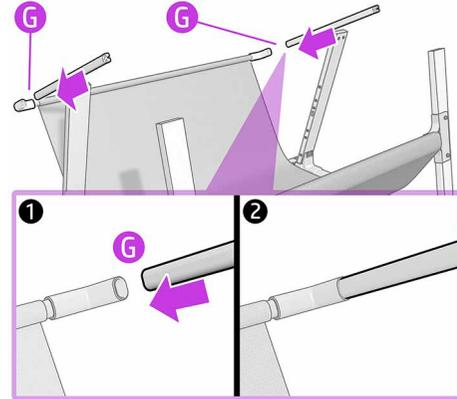
Slot the two tubes into the basket frame (G).
