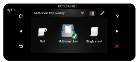
The front panel has a large central area to display dynamic information and icons. On the left and right sides you can see up to six fixed icons at different times. Normally they are not all displayed at the same time.
