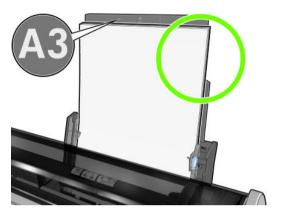
If the paper is hanging over the back of the input tray as shown, it may fail to load.
