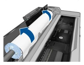
6. Reload the roll, or load a new sheet; see Paper handling on page 25.
