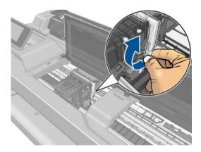
12. Remove the printhead, keeping it vertical to avoid getting ink on the connections.
