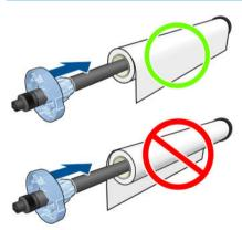
Ensure both ends of the roll are as close to the spindle stops as possible.
