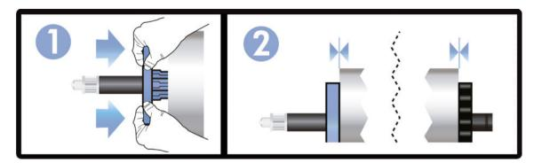
6. Ensure the blue paper stop is pushed in as far as it goes. Check that there is no space between the roll and the stops at both ends.
