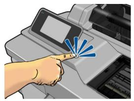
However, if you plan to store the printer for a long period or the power key does not seem to work, you are recommended to unplug the power cord.
