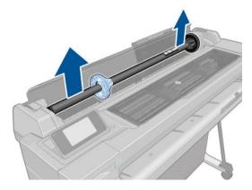
2. The spindle has a stop at each end to keep the roll in position. The blue stop can be removed to mount a new roll; it slides along the spindle to hold rolls of different widths. Remove the blue paper stop from the end of the spindle.
