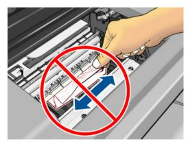
**CAUTION:** Do not move the paper sideways, as it could damage the printer.
