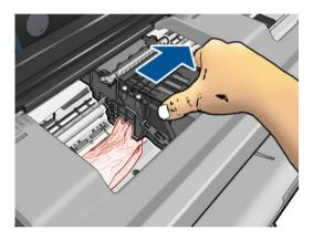
3. Carefully remove any of the jammed paper that you can lift up and out from the top of the printer.
