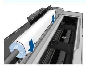
Roll the paper into the printer until you feel resistance and the paper flexes slightly. When the printer detects the paper, it beeps, and feeds in the paper automatically.
