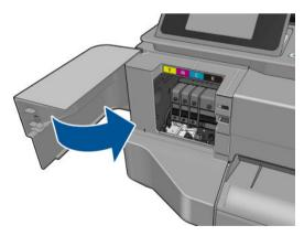
**20**. Tap **Done** on the front panel. The front panel recommends a printhead alignment.
