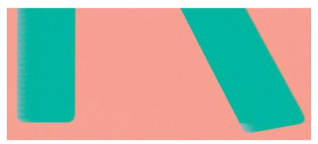
If edges of objects or lines appear to be poorly defined or lighter in density, and you have already set the print-quality slider to **Quality** in the driver dialog, select the custom print-quality options, and try setting the quality level to **Speed**. See <u>Printing on page 35</u>.
