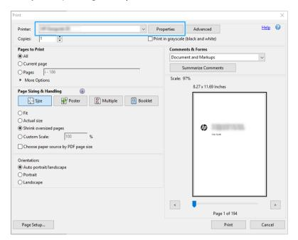
3. Adjust the color settings in the driver properties window. Click the **Properties** button in the **Print** dialog and set the **Color** option in the **Color** tab. If you have a V4 driver, check the box **Printer Managed Colors**, and select the most convenient source profile. Click **OK**.
