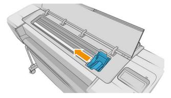
4. Carefully remove any of the jammed paper that you can lift up and out from the top of the printer.
