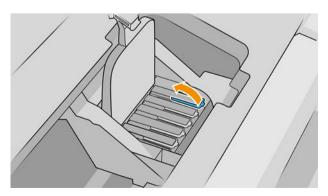
9. Using the blue handle, use steady force to disengage the printhead.
