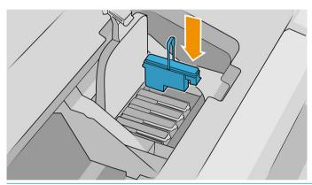
When installing the new printhead there may be some resistance, so you need to press it down firmly but smoothly. You should hear a beep and see confirmation on the front-panel display that the printhead has been inserted. If you have difficulty, see Cannot insert a printhead on page 179.
