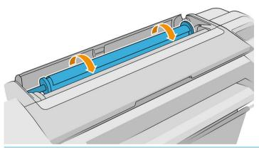
TIP: When loading the upper roll, avoid inserting roll paper into the cut-sheet slot. If you do so, the printer beeps and the front panel asks you to remove the paper.
