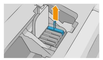
10. Pull the blue handle upward until the printhead is released from the carriage.
