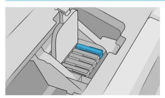
4. Insert all other printheads that need to be installed, and close the carriage lid.
