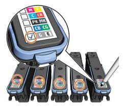
Insert the new printhead into its correct slot in the carriage.
