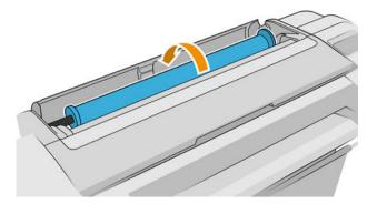
6. If the paper is stuck and cannot be rewound further, cut it from the roll.
