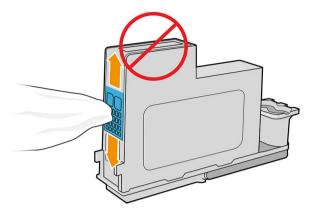
Reinsert the printhead into the same slot from which you removed it, see Insert a printhead on page 131.
