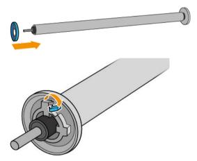
8. Load the take-up reel into the printer by pushing firmly on both ends.
