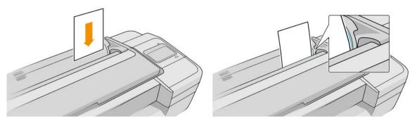
6. Load your sheet aligned with the load line and insert it until the paper will not continue; with thicker sheets, you feel resistance.
