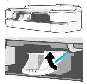
9. Remove the printhead, keeping it vertical to avoid getting ink on the connections.
