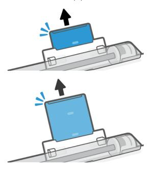
3. Load sheets of paper into the tray with the printed side facing outwards. Ensure that the sheets are all of the same size.
