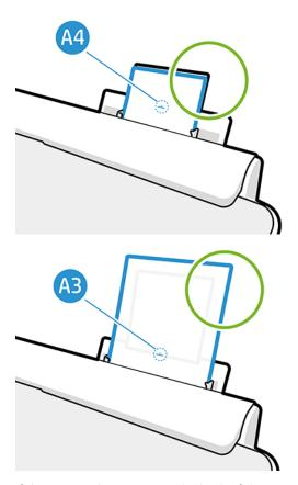
If the paper is hanging over the back of the input tray as shown, it may fail to load.
