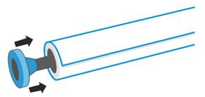
Ensure both ends of the roll are as close to the spindle stops as possible.
