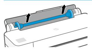
2. The spindle has a stop at each end to keep the roll in position. The blue stop can be removed to mount a new roll; it slides along the spindle to hold rolls of different widths. Remove the blue paper stop from the end of the spindle.
