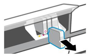
6. Insert the new ink cartridge. Make sure that you insert the ink cartridge into the slot that has the same colored letter as the cartridge you are installing.
