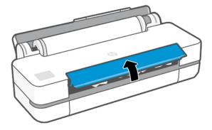
**ENWW** Paper mismatch 73 3. Rewind the roll to create a loop. Cut the paper, if needed.
