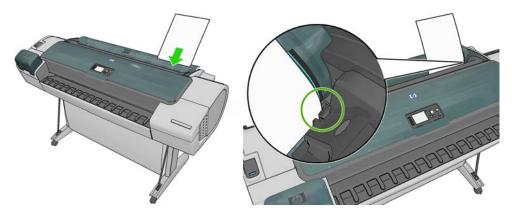
Load your sheet aligned with the load line and insert until the paper will not continue; with thicker sheets, you feel resistance.
