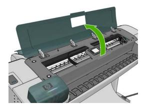
Find the printhead drop detector beside the stored printhead carriage.
