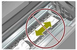
△ CAUTION: Do not move the paper sideways, as it could damage the printer.
