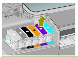
NOTE: Avoid touching the end of the cartridge that is inserted into the printer, as there may be ink on the connection.
