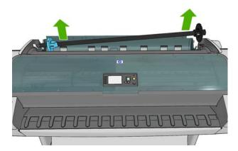
3. The spindle has a stop at each end to keep the roll in position. The blue stop can be removed to mount a new roll; it slides along the spindle to hold rolls of different widths. Remove the blue paper stop from the end of the spindle.
