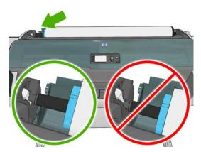
9. With both hands, push the spindle into both roll holders at the same time.
