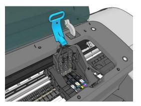
8. To remove a printhead, lift up the blue handle.
