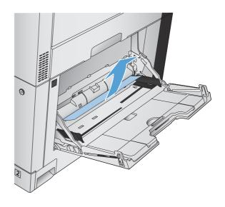
If you cannot remove the paper, or if no jammed paper is visible in Tray 1, close Tray 1 and open the right door.
