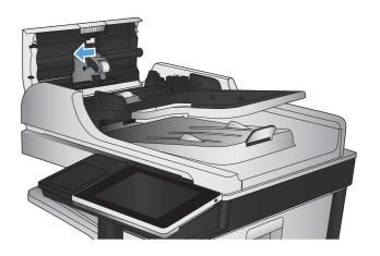
**4.** Lift the jam-access door, and remove any jammed paper.
