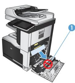
4. Paper could be jammed inside the fuser where it would not be visible. Grasp the blue handles on both sides of the fuser, and pull the fuser straight out of the product.
