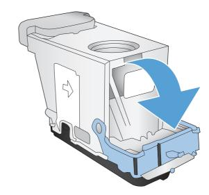
**6.** Insert the staple cartridge. Press down on the top of the staple cartridge until it clicks into place.
