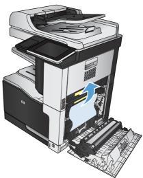
3. If paper is visible entering the bottom of the fuser, gently pull downward to remove it.
