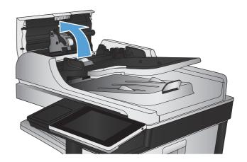
3. Remove any visible lint or dust from each of the feed rollers and the separation pad using compressed air or a clean lint-free cloth moistened with warm water.
