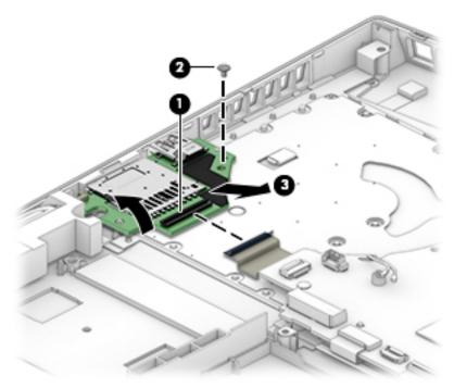
Reverse this procedure to install the card reader/USB board.
