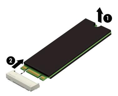
Reverse this procedure to install the solid-state drive or Optane memory module.
