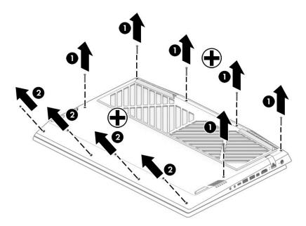
2. Insert a plastic tool between the bottom cover and the computer chassis (1), and then flex and lift the edge of the bottom cover enough to separate it from the computer (2).
