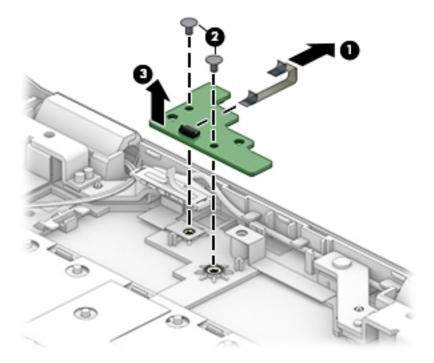
Reverse this procedure to install the thermal sensor board.
