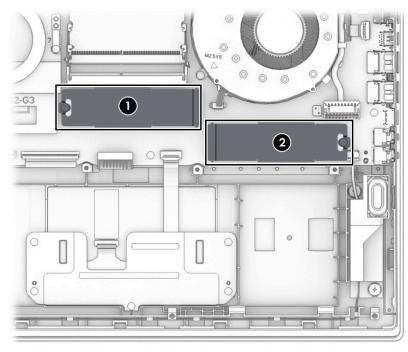
Remove the solid-state drive or Optane memory module:
