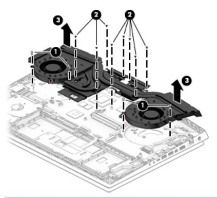
**IMPORTANT:** Thermal material must be applied on site and therefore is not included in component spare part kits. When removing any part that also requires removal of the heat sink, be sure to order and apply thermal material.
