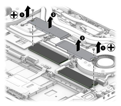
Lift the top of the drive (1), and then pull the drive from the socket (2).
