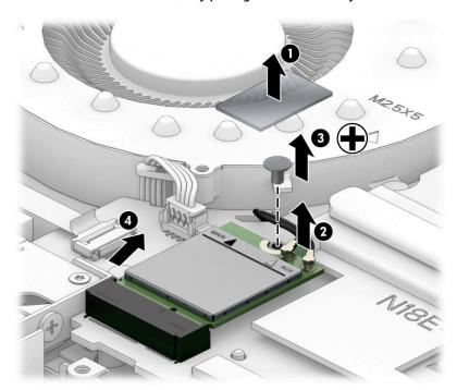
NOTE: If the WLAN antenna is not connected to the terminal on the WLAN module, a protective sleeve must be installed on the antenna connector, as shown in the following illustration.
