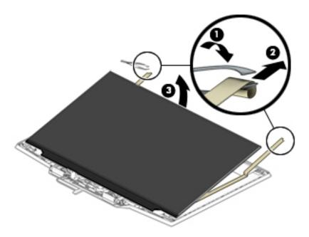
**d.** When installing the display panel adhesive tape, peel the backing from the bottom of the tape (1), and then install the tape onto both sides of the inside of the display back cover (2). Remove the backing from the top of the tape before installing the display panel (1).
