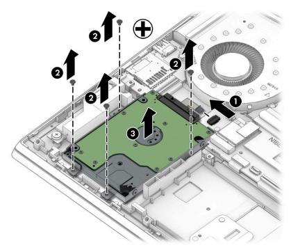
4. If it is necessary to disassemble the hard drive, remove the four Phillips M3.0 × 3.0 screws (1) from the brackets, and then remove the brackets from the hard drive (2). Disconnect the connector from the drive (3).
