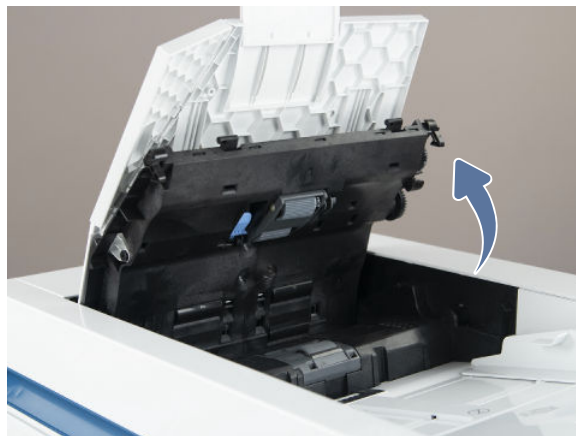
Figure 9-10 Open the document-feeder jam access door
