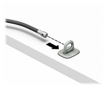
4. If your workstation configuration includes a monitor that you want to secure, pull the two scissor hands of the monitor lock apart and insert the lock into the security slot on the rear of the monitor (1), close the scissor hands (2) together to secure the lock in place, and then slide the cable guide through the center of the monitor lock (3).
