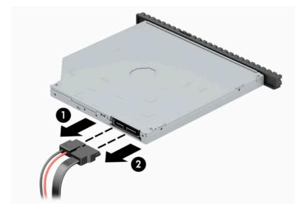
4. Press the release lever on the back of the drive (1), and then slide the drive through the front bezel (2).
