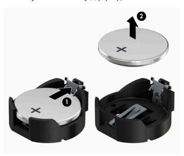
**b.** To insert the new battery, slide one edge of the replacement battery under the lip of the holder with the positive side (1) sup . Push the other edge down until the clamp snaps over the other edge of the battery (2).
