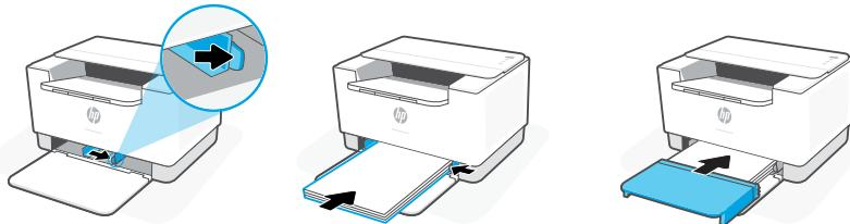
**EN** Slide out the guides. Load Letter or A4 paper and adjust the guides. Slide the tray cover into place.
