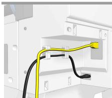
Route the Ethernet cable and power cable though the cable clips.
