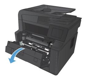
3. Remove the jammed sheet by pulling it straight out.
