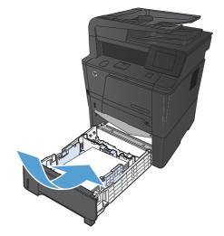
5. Push down on the paper to make sure that the paper stack is below the paper limit tabs at the rear of the tray.
