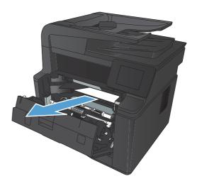
4. Reinstall the print cartridge, and then close the print cartridge door.
