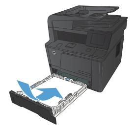
Push down on the paper to make sure that the paper stack is below the paper limit tabs on the right side and rear of the tray.
