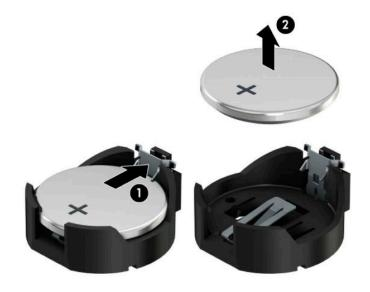
**b.** To insert the new battery, slide one edge of the replacement battery under the lip of the holder with the positive side up (1). Push the other edge down until the clamp snaps over the other edge of the battery (2).
