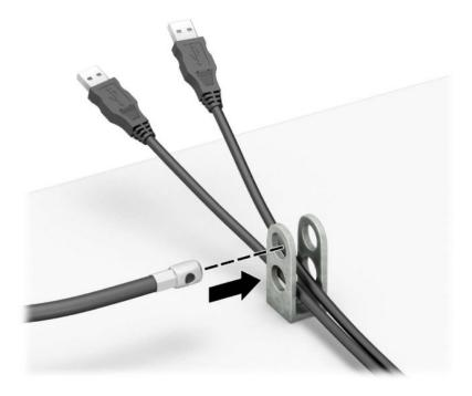
8. Remove the thumbscrew from the rear of the chassis and screw the lock to the chassis in the thumbscrew hole.
