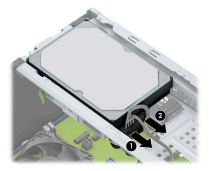
7. Remove the mounting screws (1) and pull the drive up and out of the cage (2).
