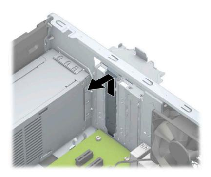
**b.** If you are removing a PCI Express x1 card, hold the card at each end and carefully rock it back and forth until the connectors pull free from the socket. Lift the card straight up (1) then away from the inside of the chassis (2) to remove it. Be sure not to scrape the card against other components.
