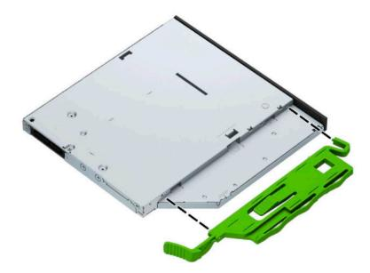
9. Slide the optical drive through the front bezel (1) all the way into the bay so that the green latch locks onto the chassis frame (2).
