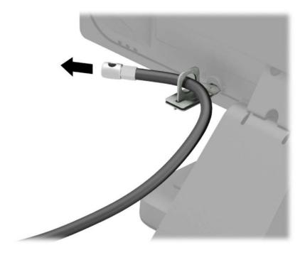
6. Attach the accessory cable fastener to a desktop using the appropriate screw for your environment (screw not provided) (1), and then place the accessory cables into the base of the fastener (2).
