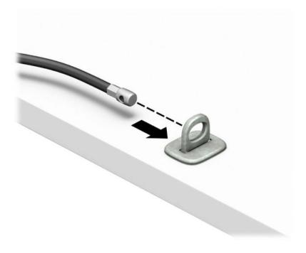
Pull the two scissor hands of the monitor lock apart and insert the lock into the security slot on the rear of the monitor (1), close the scissor hands together to secure the lock in place (2), and then slide the cable guide through the center of the monitor lock (3).
