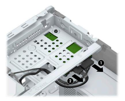
7. Remove the three 6-32 mounting screws (1) and slide the drive out of the bay (2).
