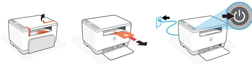
**EN** Remove all tape and pull the paper sheet from the printer. Plug in and turn on the printer.
