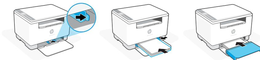
**EN** Slide out the guides. Load Letter or A4 paper and adjust the guides. Slide the tray cover into place.
