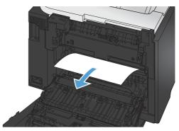
4. If you can not see any jammed paper, lift the duplexing unit using the tab on the side of the duplexing unit.
