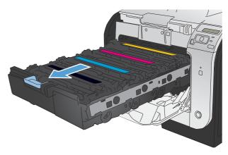
3. Grasp the handle on the old print cartridge and then pull the cartridge straight up to remove it.
