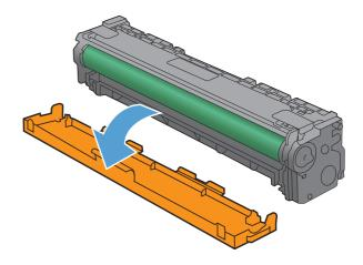
Do not touch the imaging drum on the bottom of the print cartridge. Fingerprints on the imaging drum can cause print-quality problems.
