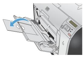
4. Extend the paper guides fully (callout 1) and then load the paper stack into Tray 1 (callout 2). Adjust the paper guides to the size of the paper.
