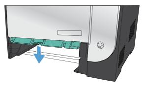
4. Remove the jammed sheet by pulling it straight
