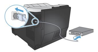
2. Wait for 60 seconds before continuing. During this time, the network recognizes the product and assigns an IP address or host name for the product.
