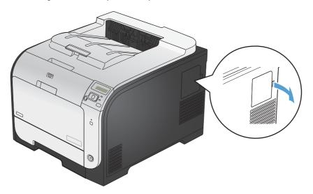
3. Remove the DIMM access door.
