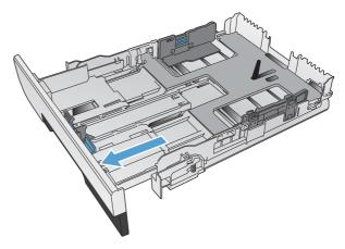
4. Place the paper in the tray and make sure that it is flat at all four corners. Slide the side paper width guides so that they align with the papersize marking in the bottom of the tray. Slide the front paper length guide so that it pushes the stack of paper against the back of the tray.
