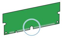
Holding the DIMM by the edges, align the notch on the DIMM with the bar in the DIMM slot at an angle.
