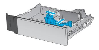
Load paper into the tray. Check the paper to verify the guides lightly touch the stack, but do 3. not bend it. For information about how to orient the paper, see Table 2-2 Tray 2 and the 500sheet trays paper orientation on page 21.
