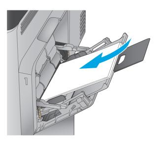
4. Make sure that the paper fits under the fill line on the paper guides.
