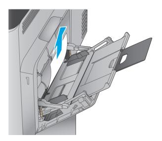
2. If you cannot remove the paper, or if no jammed paper is visible in Tray 1, close Tray 1 and open the right door.
