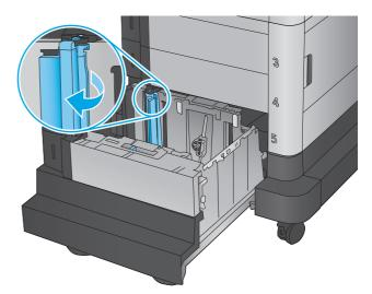
4. Load paper into the tray. Check the paper to verify the guides lightly touch the stack, but do not bend it.
