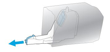
5. Insert the bottom of the new unit into the product first and then push the top of the unit until it clicks into place.
