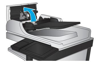
Remove any visible lint or dust from each of the feed rollers and the separation pad using compressed air or a clean lint-free cloth moistened with warm water.
