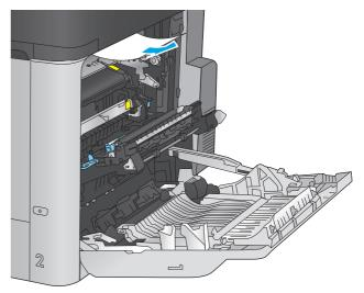
12. Paper could be jammed inside the fuser where it would not be visible. Grasp the fuser handles, lift up slightly, and then pull straight out to remove the fuser.
