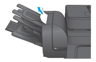
2. Lift the gray latch on the front of the stapler, and open the stapler cover.
