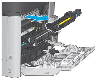
**13.** Open the jam-access door. If paper is jammed inside the fuser, gently pull it straight up to remove it. If the paper tears, remove all paper fragments.
