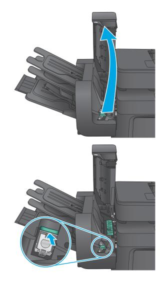
3. Insert the new staple cartridge into the stapler and push down on the green handle until it snaps into place.
