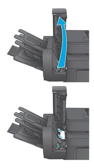
3. If jammed paper is visible underneath the paper guide, pull it straight out.
