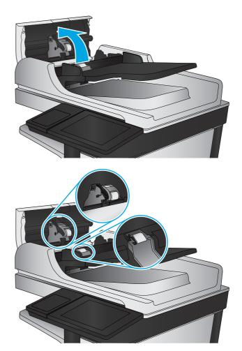
3. Remove any visible lint or dust from each of the feed rollers and the separation pad using compressed air or a clean lint-free cloth moistened with warm water.
