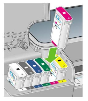
4. Push the cartridge into the slot until it snaps into position. You should hear a beep and see confirmation that the cartridge has been inserted.
