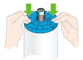
Ensure the blue paper stop is pushed in as far as it goes; until both ends are against the stoppers. 7.
