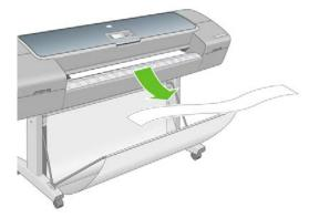
The sheet stays in the printer when the print has been completed 155
