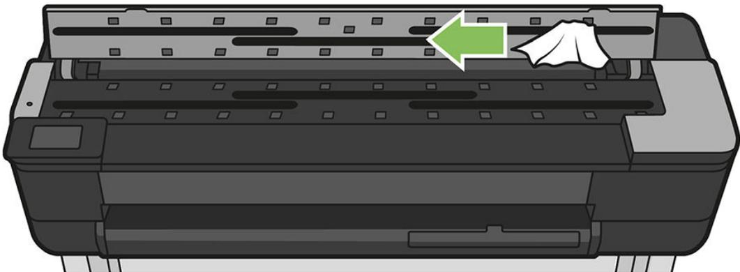
5. For more thorough cleaning, clean the calibration surfaces and the feed rollers.
