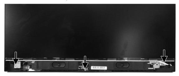
**10.** From the rear of the computer, remove the four Phillips screw located along the bottom edge of the computer.
