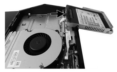
8. Disconnect the power and data cables from the hard drive. There is a tab you can pull to disconnect these cables.
