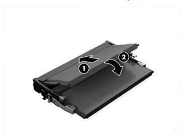
NOTE: A memory module can be installed in only one way. Match the notch on the module with the tab on the memory slot.
