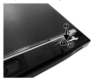
9. Remove the power button board from the computer.
