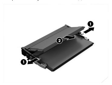
5. Slide the new memory module into the slot at approximately a 30° angle (1), then press the memory module down (2) so that the latches lock it in place.
