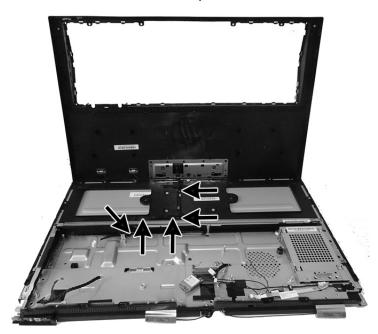
13. To remove the main chassis, remove the four Phillips screws around the sides (1) and the Phillips screw in the middle (2) of the chassis.
