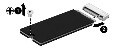
To install the solid-state drive, reverse the removal procedures.
