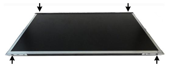
**12.** Pull the brackets off the sides of the display panel.
