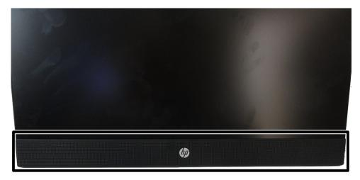
5. Rotate the top of the cover downward to disengage the snaps from the chassis, and then remove the cover.
