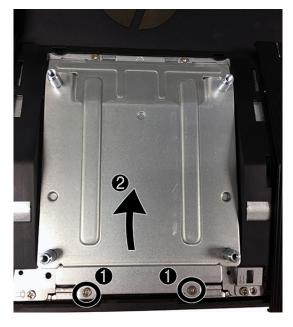
To install a VESA bracket, reverse the removal procedures.
