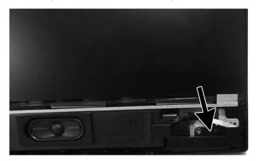
**7.** Remove Phillips screw **(1)** that secures the power button board to the computer.
